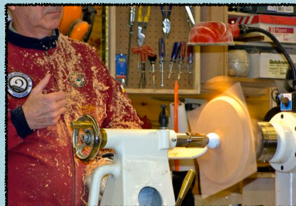
THE WINGS HAVE TO BE TURNED FIRST and the outer edges near the points needs to be super glued and taped to stop chipping out in that area.
