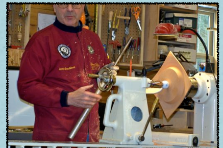
THE BOWL ON TOP OF THE WINGS must match the bowl shape on the bottom. The edge thickness needs to be uniform & may have to be corrected when the tenon is removed.
