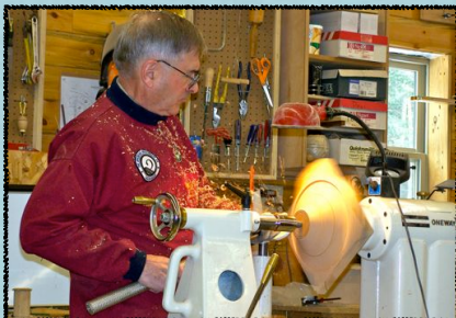
STARTING THE BOTTOM and shaping the wings and the bowl shape keeping the bowl shape within the wings No sanding at this point.
