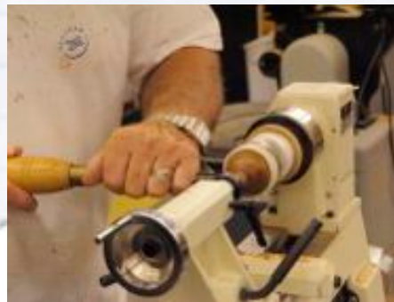
CUTTING THE 1/2 INCH NIPPLE USING THE PVC PIPE CHUCK.
