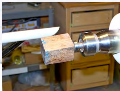
THE BOTTLE STOPPER BLANK SCREWS ONTO THE THREADED SHAFT AGAINST THE STOP.
