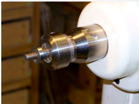
TIM SHOWED AN EXAMPLE OF A BOTTLE STOPPER CHUCK. IT IS HELD IN A COULET CHUCK.
